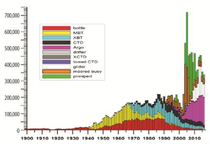
Number of subsurface ocean temperature profiles per year by instrument type 1900-2017. [MBT=Mechanical Bathythermograph, XBT=Expendable Bathythermograph, CTD=Conductivity-Temperature-Depth, XCTD=Expendable CTD.]
